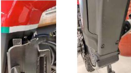
Then insert a 4 mm wrench in the specific socket head screw and turn it clockwise one-fourth of a turn to make the battery come down. At this point, press the chrome-plated tab downwards with your finger in order to completely remove the battery.
