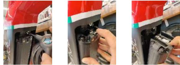
To install the battery: match the protrusion of the bottom support with the groove found on the bottom of the battery and, while pivoting on the lower base, accompany the upper part of the battery inside the frame.
